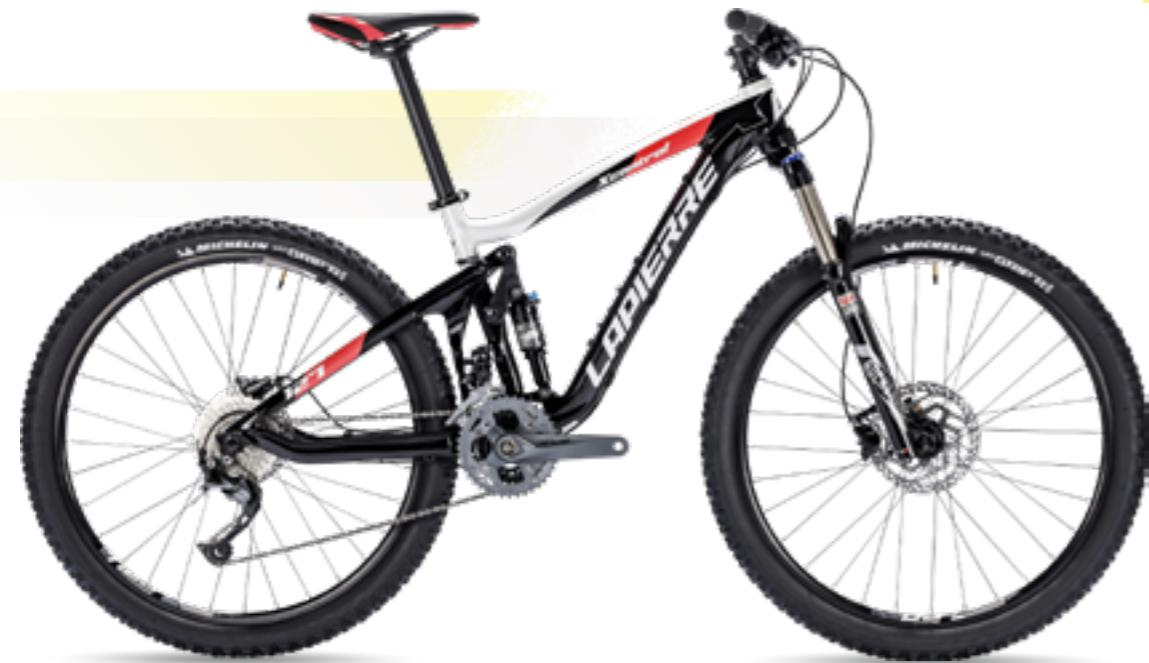
X-CONTROL 27.5" SUPREME 6 ALLOY FPS+ 100mm travel PRESSFIT THRU AXLE 12x142
