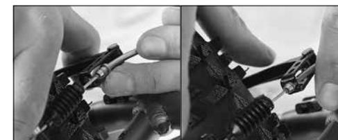
3. b) Hydraulic rim brakes: fitting is as removal only in reverse sequence.
