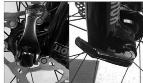
3. Open the quick-release thru axle to remove it. After opening the lever, you can unscrew the thru axle and remove it completely from the hub.
