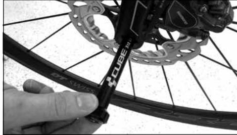
2. Use a hex wrench to hand tighten the thru axle.
