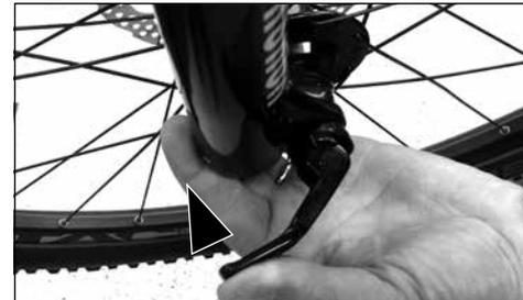
Ensure that the lever is tight and that the clamping lever is positioned correctly. Please see the operating manual from your thru axle manufacturer for the correct position and setting.
