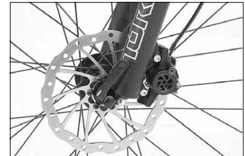
**1. Pull the brake caliper alternately in all directions.**
