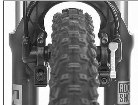
**1. Check that the entire brake system is secured and screwed in correctly:**
