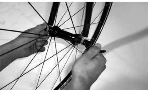
**b) To assemble the front wheel**
