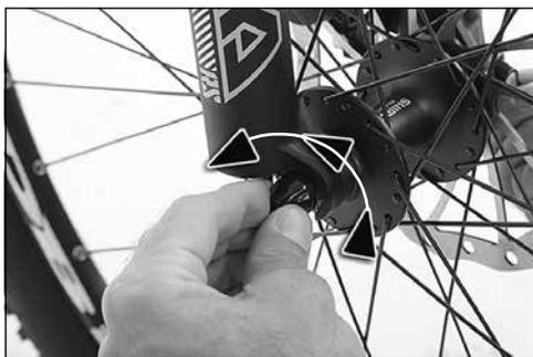
3. On saddle stem quick release levers: To loosen, instead of the nut, turn the bolt with the Allen key head itself counter-clockwise.
