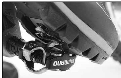
c) When the hook nose is positioned correctly in the pedal, push the whole surface of the foot sharply downwards until the clamping mechanism clearly and audibly engages.
