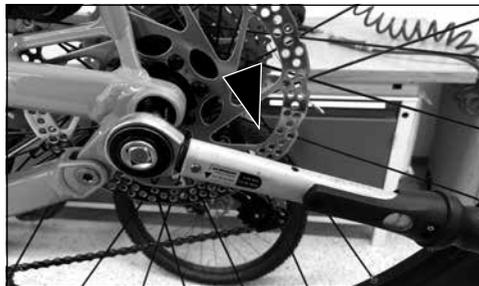
4. To remove the thru axle, you must unscrew it using a hex wrench.
