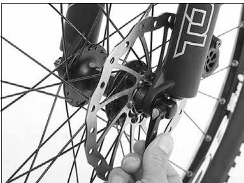
2. Turn the nut counter-clockwise until the wheel can be removed from the frame or front forks without any great effort.
