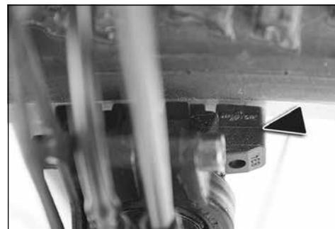
**4. Check the brake block wear.**
