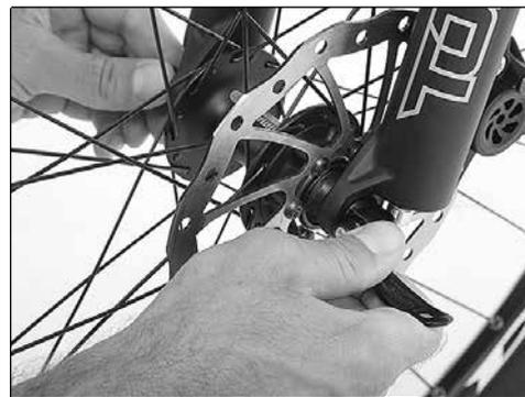
5. Now turn the nut or the Allen key bolt head until the excentric lever, when turned around its bearing more than 90° to meet slight resistance (it now forms an approximately straight line extension of the hub axis).
