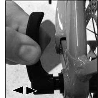
3. Releasing the RWS clamping lever, it will securely lock into the desired position. Please ensure that the lever is tight and the clamping lever is positioned correctly. Please double check the manual of your thru axle manufacturer for the correct positioning and setting.
